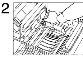
Use the enclosed cleaner to clean the fixing roller.
