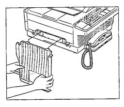
**Caution:** Do not pull open the holder strongly since it is out of place. Install the receiving tray by inserting tabs of the tray into slots in the paper ejection area of the unit.
