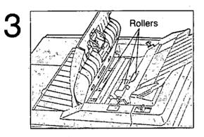
Open the document feeder unit by pressing the latch button.
