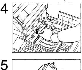
Insert the fixing roller cleaner.
