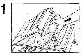
Open the cover and remove the supply cartridge.
