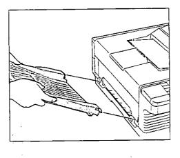
Install the receiving tray on the left side of the unit by inserting tabs of the tray into holes on the unit.
