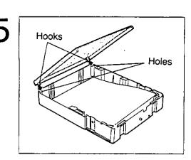
Replace the paper cassette cover. Be sure that the cassette cover hooks are in the holes of the cassette case.
