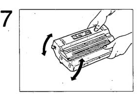
Gently rock the supply cartridge 5 or 6 times at a 45 angle.
