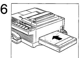
Insert the paper cassette into the unit until it is firmly in place.
