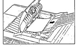
Close the document feeder unit carefully by pushing down until the cover locks into position.
