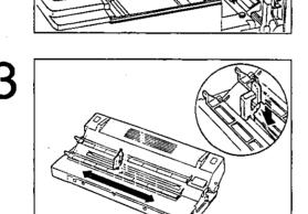
Attach it securely to the cartridge's guide rail and clean the primary corona wire. Be sure to return the cleaner to its storage location after use.
