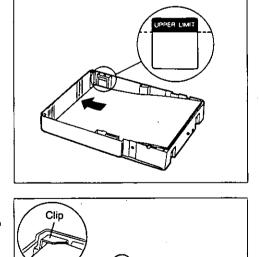
Push the paper under the clips. Be sure the corners of the paper are inside the cassette.
