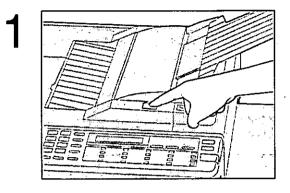
Press the latch button to open the document feeder unit.
