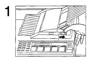
Slide the door open lever to open the cover of the unit.
