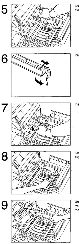
Use the new fixing roller cleaner to clean the fixing roller.
